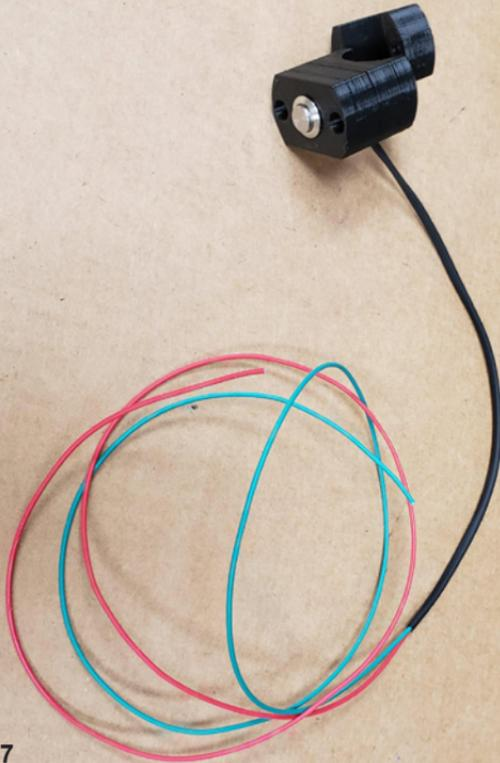
All METrans Vehicles are equipped with a manual horn button on the Vehicle dashboard. The horn on the METrans Vehicle is activated in two ways: First, via the manual, momentary horn button on the vehicle dashboard. Second, automatically, via the laser activated Operator Safety System.
