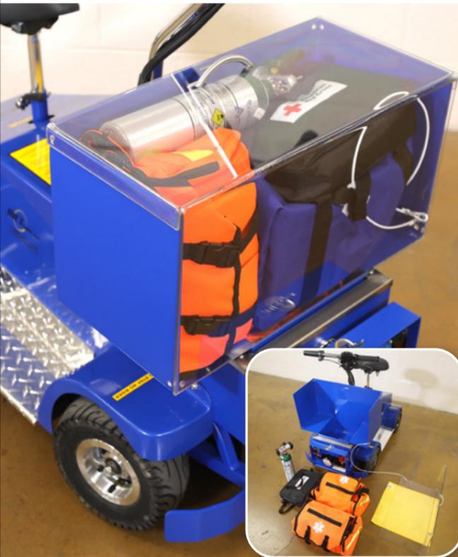
All METrans Vehicles are equipped with a Stainless-Steel Front Cargo Bin. One customer has specified the use of the METrans MT700.01 Vehicle as a Paramedic and EMT first responder vehicle due to its size, speed and maneuverability.
