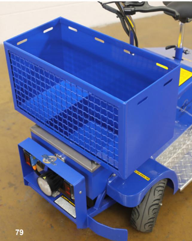
All METrans Vehicles are equipped with a Stainless-Steel Front Cargo Bin. Some customers have observed the standard equipment cargo bin is too small to accommodate their needs.
