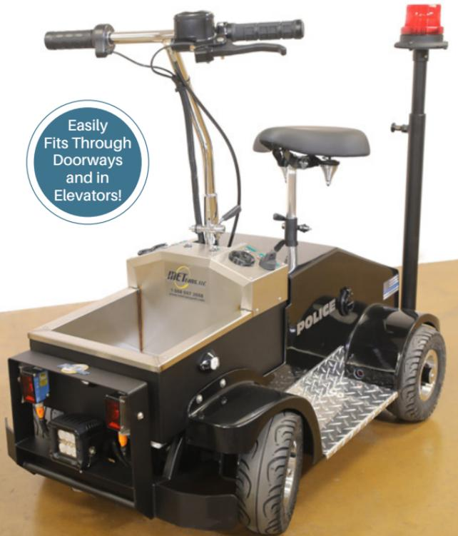
The **Micro Police Interceptor (MPI)** is a fast, dedicated, highly maneuverable, small-format Vehicle that can quickly reach a top speed of +/-14MPH. The optional **MPIT Cart/Trailer** adds easy, functional transport of additional equipment and supplies.
